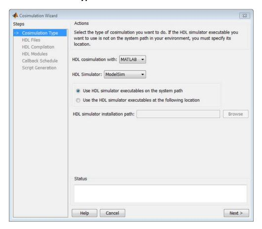
On the Cosimulation Type page, you select options that determine whether a function or block is to be generated and for which HDL simulator.
