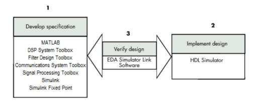
As the figure shows, EDA Simulator Link software connects tools that traditionally have been used discretely to perform specific steps in the design process. By connecting these tools, the link simplifies verification by allowing you to cosimulate the implementation and original specification directly. This cosimulation results in significant time savings and the elimination of errors inherent to manual comparison and inspection.
