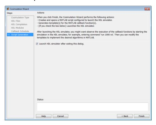
The Cosimulation Wizard now has all the information it needs to generate an EDA Simulator Link component or test bench function.
