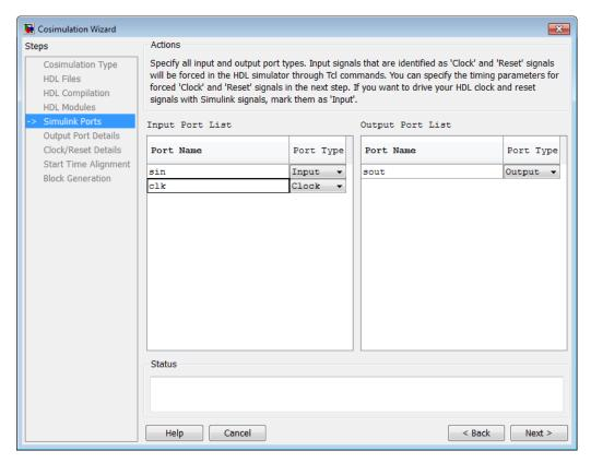
On the **Simulink Ports** page, you specify the type of each input and output port. The Cosimulation Wizard attempts to determine the port types for you, but you may override any setting.
