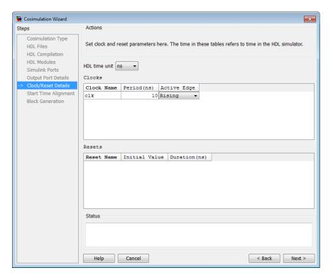
On the **Clock/Reset Details** page, you set the clock and reset parameters. The time period specified here refers to time in the HDL simulator.
