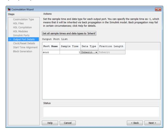
On the **Output Port Details** page, you set the sample time and data type for all output ports.
