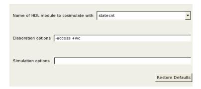
On the **HDL Module Selection** page, you provide the name of the HDL module to be used in cosimulation.
